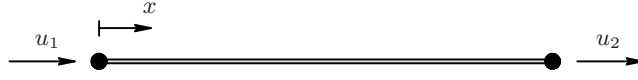
Figure D.3: A beam element with the sign convention for longitudinal vibration.
