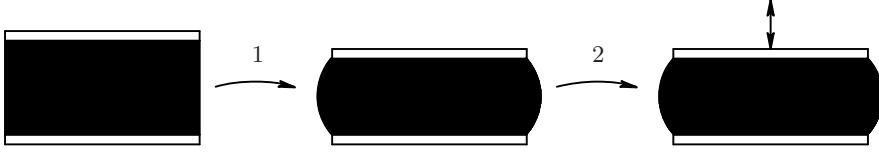
Figure 5.2: Analysis procedure for rubber vibration isolators: the first step is the calculation of the static pre-deformation (1) and the second step is the superposed harmonic analysis (2).
