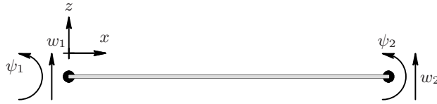
Figure D.2: A beam element with the sign convention for bending vibration.
